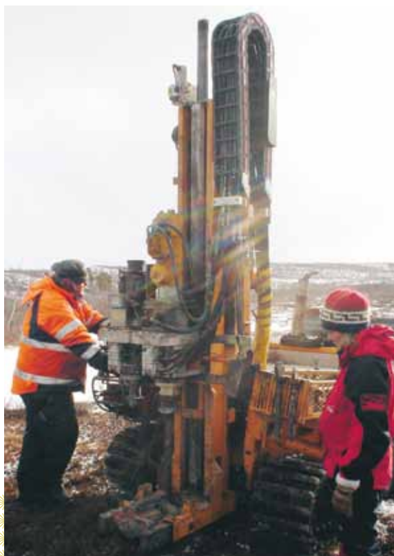
New holes are drilled for measurements of ground temperature in the vicinity of Abisko Research Station. Drilling is supervised by researcher Margareta Johansson, Lund University. Photo: Frida Keuper
