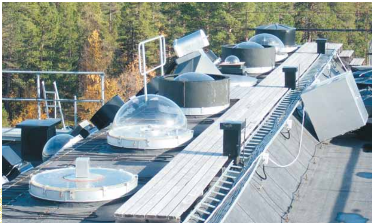
Instruments including a mm-wave radiometer and FT-IR and DOAS spectrometers are deployed on the roof of the optical laboratory at the Swedish Institute of Space Physics, IRF, in Kiruna. Photo: Rick McGregor, IRF
